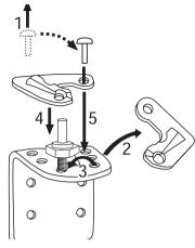
Remove the door fitting on the lower right (1) and reposition the door bearing cover from the lower left to the right of the door (2), place the door fitting supplied in the lower left of the door (3). Carefully remove the door to the front and place on one side.
